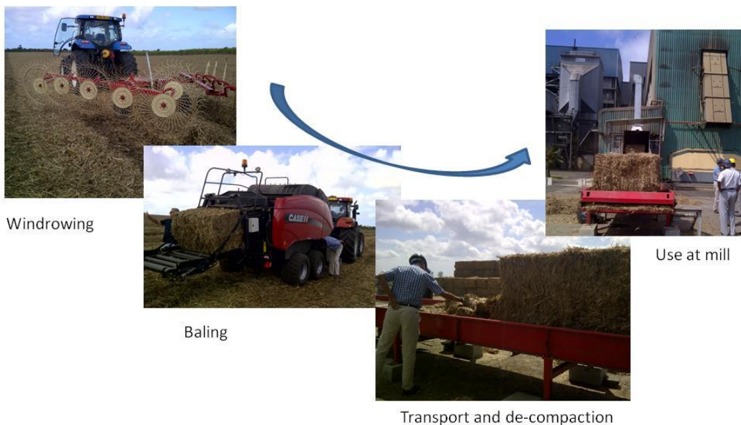
Figure 7-1: Trash collection, baling and use as bagasse mix for electricity production in Mauritius
