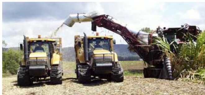
Figure 7-2: Harvester-mounted trash shredder and collection
